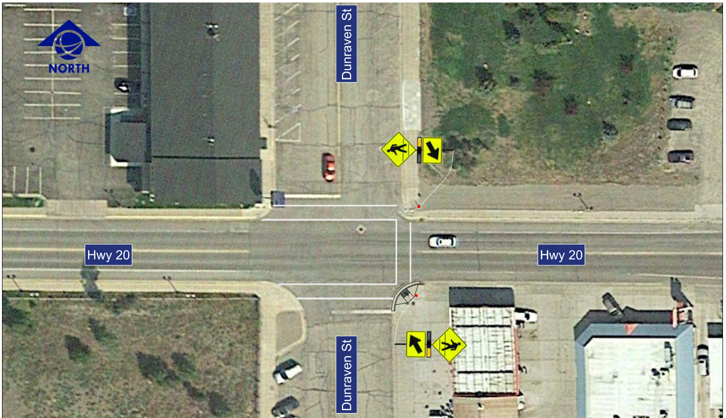
Figure 23: Concept design of crosswalk with Rapid Rectangular Flashing Beacon at Highway 20 and Dunraven Street
