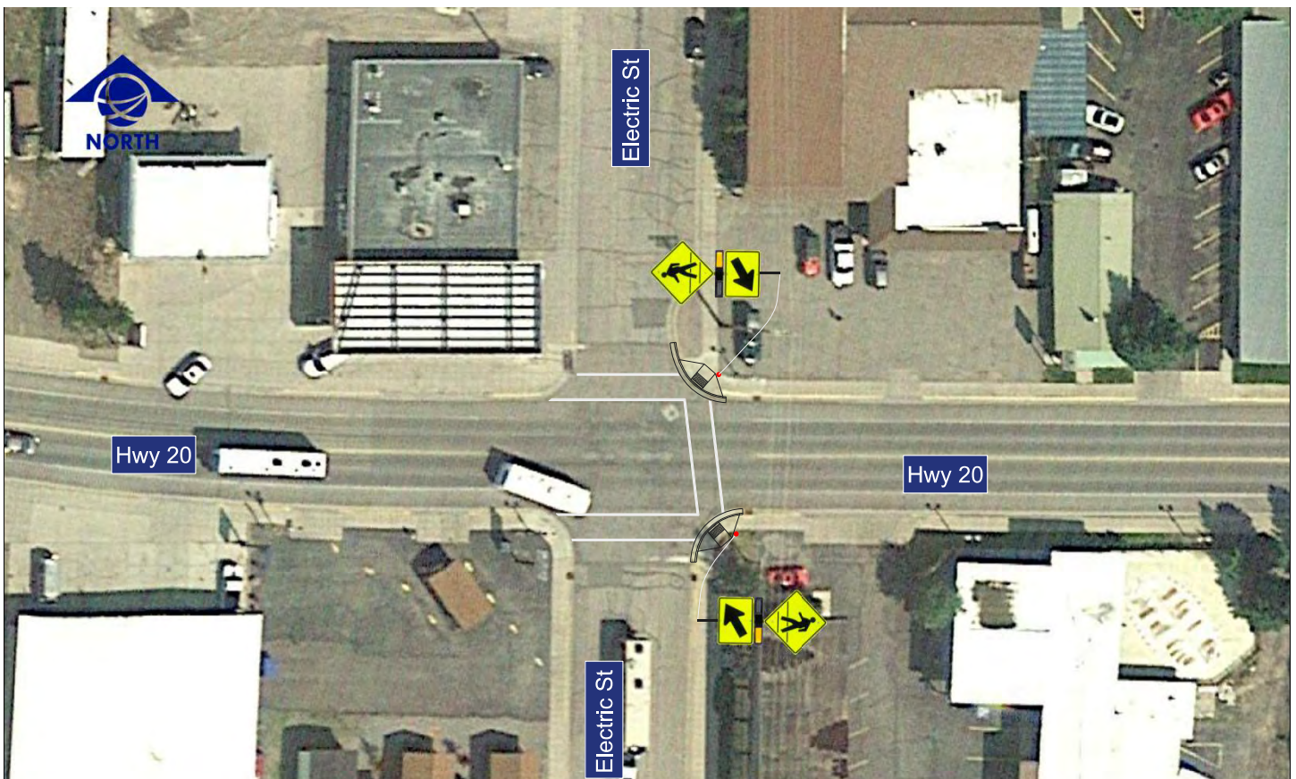
Figure 24: Concept design of crosswalk with Rapid Rectangular Flashing Beacon at Highway 20 and Electric Street
