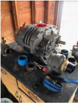
Extra blower that was sitting outside in weather. Needs to be rebuilt before installation.
